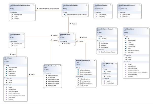
Note: The domain model consists of classes that make up the contracts with the external system. The contracts are defined as classes instead of interfaces to allow the model to be easily extended later if needed. This follow the best practice guidelines defined in the book Framework Design Guidelines.
